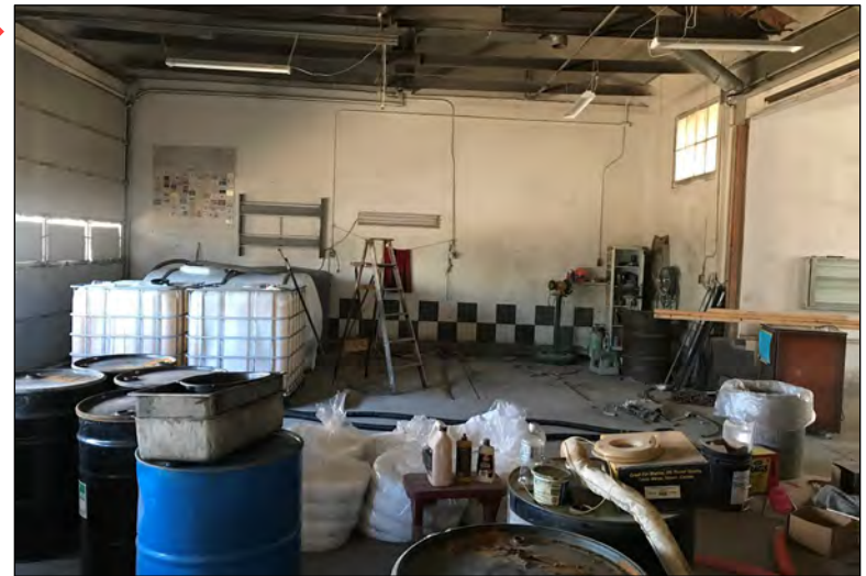
Photo 8: Inside of garage. Tanks and drums used to contain water pumped from groundwater interceptor trench until disposal at licensed facility.
